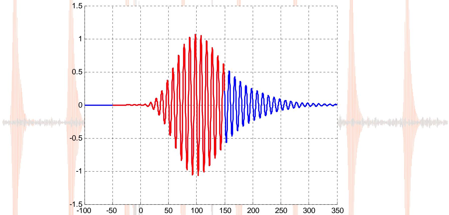
If a (certain area of a) Loran pulse is hit by a noise spike, we blank the complete Loran pulse
